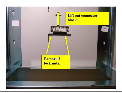
• Remove 2 lock nuts from male connector block on rear panel and lift connector block from its temporary locating holes in rear panel.
