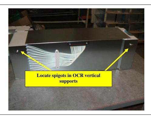
• Locate the 2 spigots on the rear of the Sub Rack into the keyhole slots in the OCR rack left and right-hand vertical supports.
