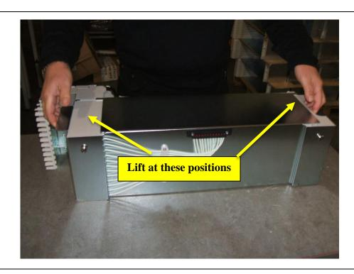
• Remove OCR Sub Rack Assembly (1) from packaging, using lifting positions as indicated.
