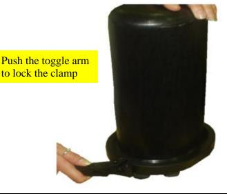
Squeeze the clamp together and engage the toggle arm. Push the toggle arm into the clamp to lock and seal.
