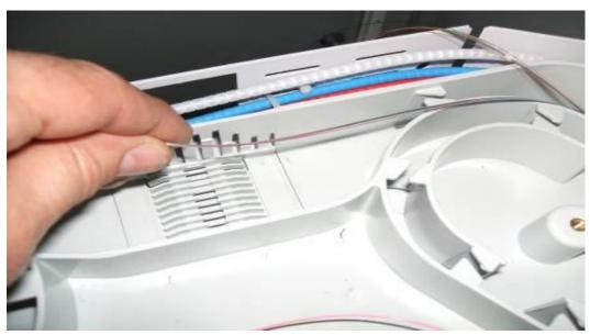
• Select the 12 Primary Coated Fibres from the BLUE tube (Fibres 1 to 12).
