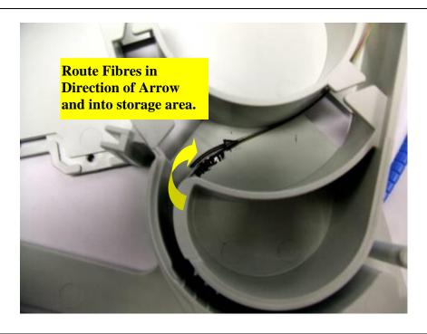
• Route the 12, fibres from the BLUE Tube in direction of Arrow.
