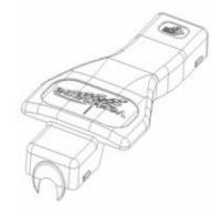
FOR 24 AND 48 FIBRE VERTICASA CABLES, BREAK OFF THE END DUST COVER USING A PAIR OF LONG NOSE PLIERS
