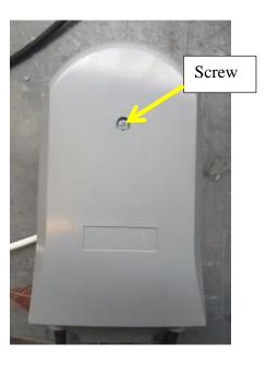
• Screw the screw tightly into the base and add the screw cover to hide the screw head.
