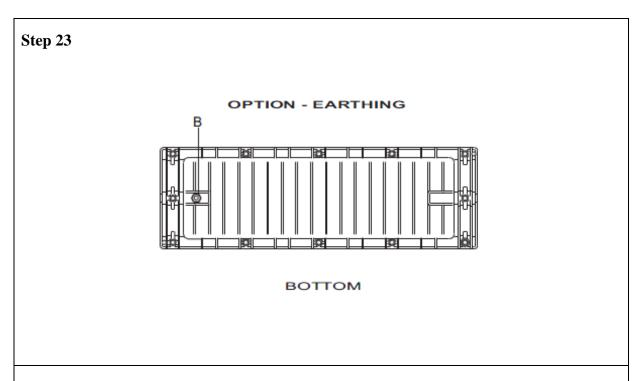
It is possible to earth cables with a metallic strength member by running a length of earth wire from the cable bracket (beneath the screw) to the earthing post of the joint located on the bottom of the joint and shown opposite by the letter B.
