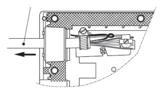
To remove a cable, slip the seals along the cable using grease if required.
