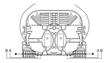
Open the two hinged locking plates on the tube entry ports and enter the fibre as shown by the arrows.
