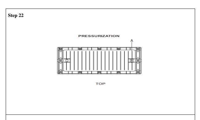
Unscrew the valve cap A. Using a foot pump and a manometer pump the joint up and bleed down to 0.4 bar.
