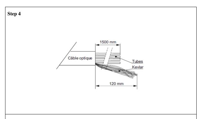
Mark the position of the cable butt at the port of the closure and strip the external sheath from the cable to expose 1500mm of the cable tubes. Cut away any excess cable length.
