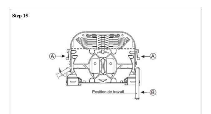
Screw the two brackets into the joint chassis and keep them lined up in the working position indicated opposite.
