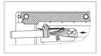
Insert the tabs of the clamping shoe on the bracket into the square holes in the joint chassis. Pull back in the direction shown in the picture to the left.
