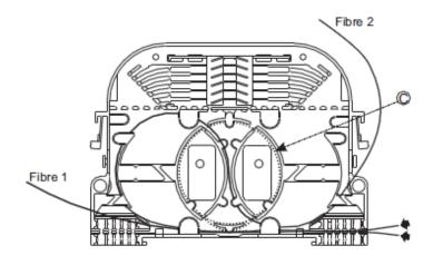
In cases where fibres enter from the same side of the tray, route one of the fibres through the central mandrel channel of the tray to change the routing direction.
