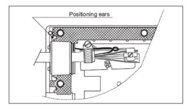
Slip the seals along the cable and seat them into position in the closure body. Ensure that the ears on the seal fit properly within the corresponding cut-outs in the flat seal.
