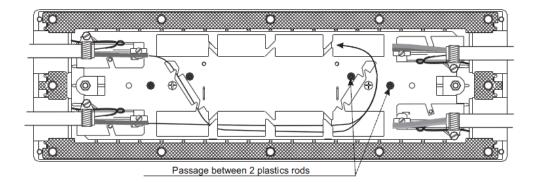
It is possible to route the bare fibres from the cable tubes through the chassis and directly onto the splice tray. When using this method, the fibres can be vulnerable to damage so extreme care should be taken.
