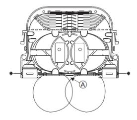
Coil the fibre length around the central storage area of the splice tray ensuring that all the fibres are fully retained beneath the routing tabs of the splice tray.
