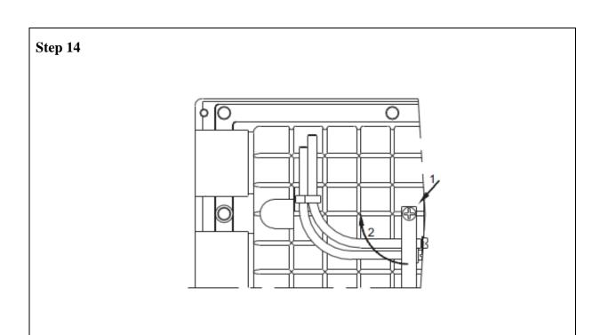
To access different cassettes to enable the routing of fibres onto the splice trays remove the two curved brackets supplied with the joint.
