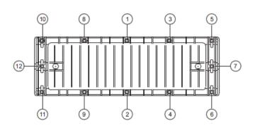
Check that all cable entry seals are correctly located and that the ears of the seals are located within the cut-outs of the flat gasket seal.
