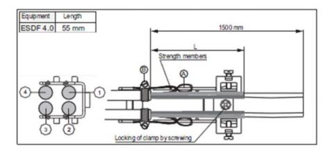
Cut the central strength members to 55mm and secure into bracket as shown.
