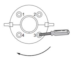
Tighten the seals in the order shown on the diagram opposite. Execute a maximum of two turns per screw before moving to the next screw.
