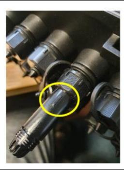
• Line the rib on the shroud body to face forwards as shown.
