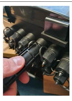
• Using the supplied port tool remove the cap from the relevant port on the Flexibox.
