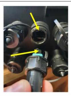
• Push MPO connector into the adapter. Ensure the pin on the MPO lines up with the pin on the MPO adapter on the box.
