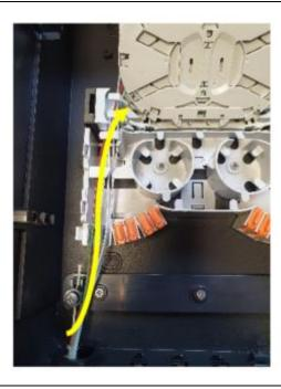
• Remove the orange retention clips from the manifold and route the fibres onto the splice tray as required.
