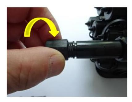
• Tighten the clamp nut ensuring the seal is in the end of the shroud.
