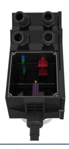
The FTTA Hybrid junction box is an aerial enclosure designed to take a single incoming preterminated hybrid cable and redistribute to up to 4 Hybrid RRH jumper cables. The box comes preconfigured ready for fibre and power connections in the access compartment and external hybrid connections. The box comes with a pole mounting kit or wall mounting bracket which allows easy, secure mounting to a mast, pole or wall.
