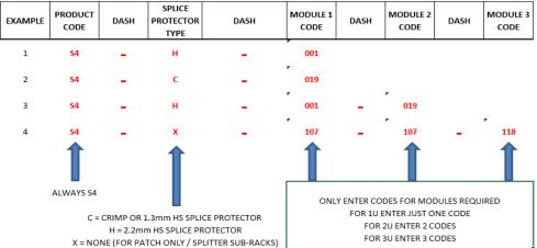
Example 1 above is for a 1U SRS Sub-Rack. The part number is S4-H-001. This denotes a 1U high SRS4000 Sub-Rack fitted with a blank Splice and Patch module. The sub-rack is for use with 2.2mm heat shrink splice protectors.
